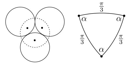
The three touching points on the central sphere will form a  $\frac{\pi}{3}$ -equilateral spherical triangle with area  $\Delta_{\frac{\pi}{3}}$ , where:
